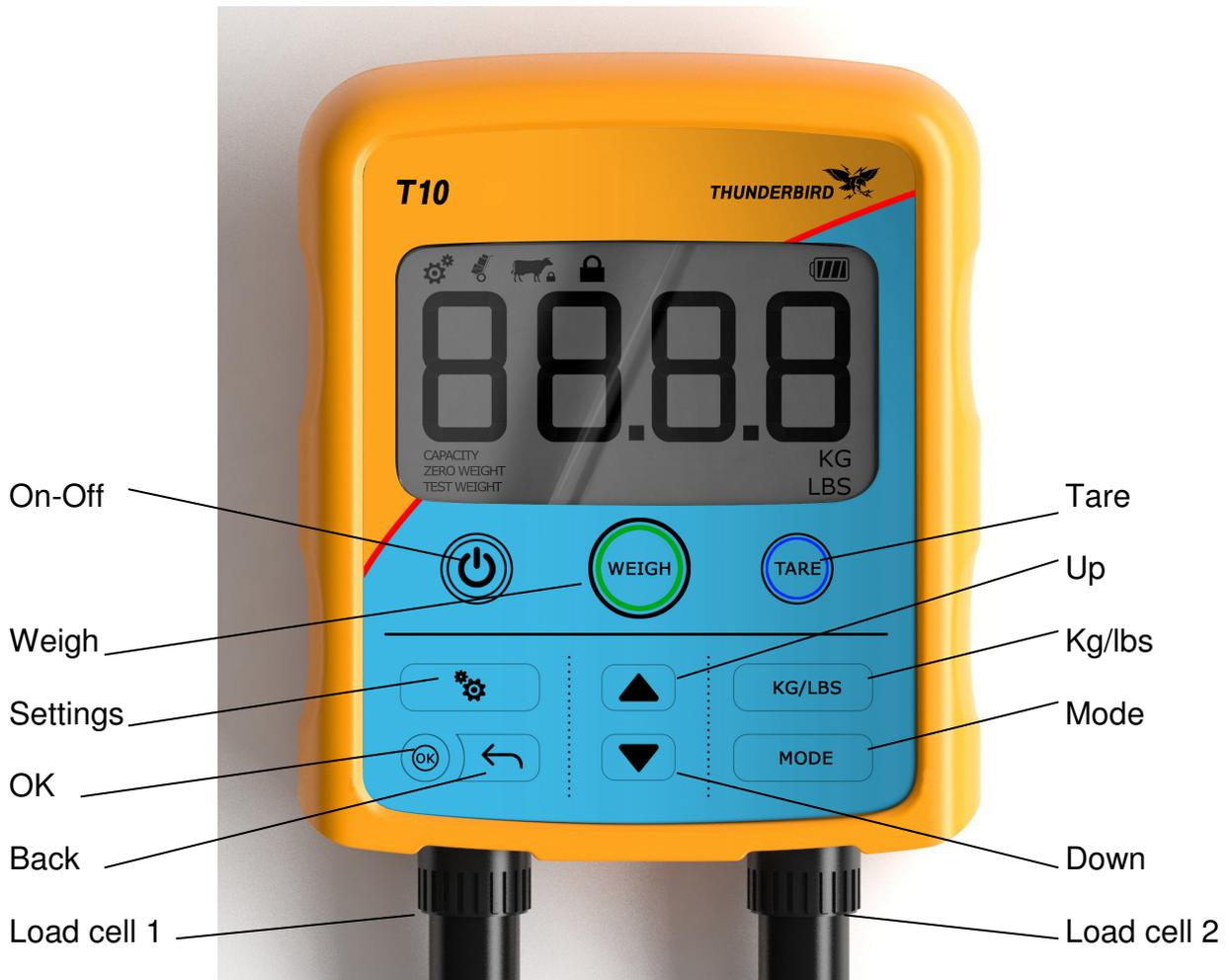
The T10 has a water resistant 10 button keypad for a user interface. An extra large 40mm digit display provides the user with the ability to view the weight at a distance. The display also has other indications that are used at various times. All mode settings and changes are memorized at the time of change, so that the indicator will return to the previous set up when it is turned on.
