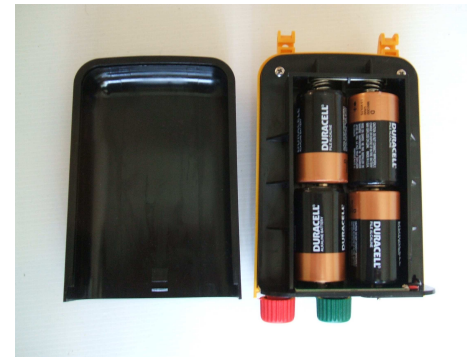
Rear plastic cover with batteries fitted
